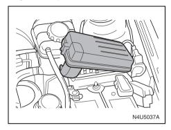
The engine compartment fuse block is located on the driver's side of the vehicle, near the battery. See "Engine Compartment Overview" in this section for more information on location.
